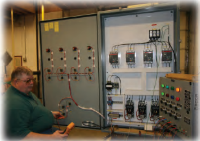
Testing a Quadruplex Panel for a Deaerator in our Controls Group Clean Room
