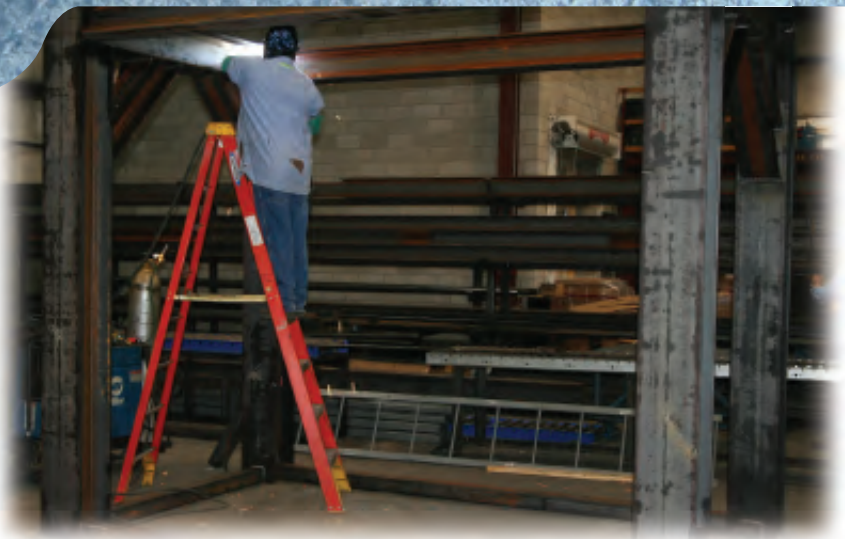
Welding a Seismic Designed Deaerator Structural Support Stand
