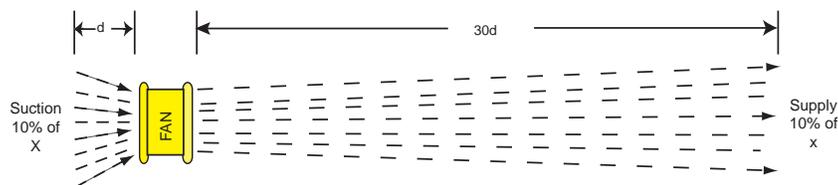
Air velocity is reduced as the distance from the fan increases on both the inlet (exhaust) and outlet (delivery) sides. However the rate of reduction in air velocity is significantly greater on the inlet side of the fan.
