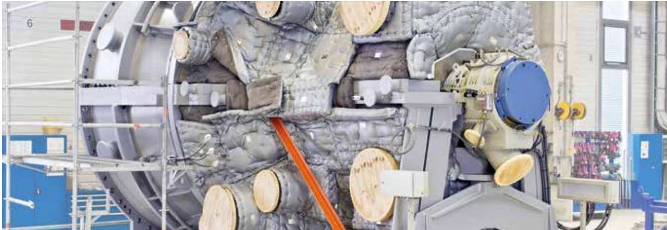
Steam turbine SST-900 for the CSP-plant NOOR III, Morocco
