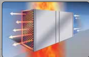
Tubular air pre-heater, typically used for very high flue gas temperatures, up to 1,750 degrees F.
