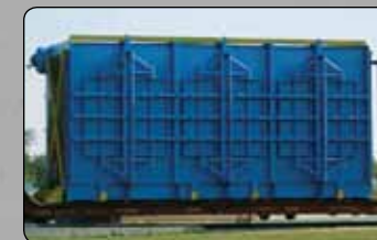
MSW boiler equipped with large Davit doors for easy access.
