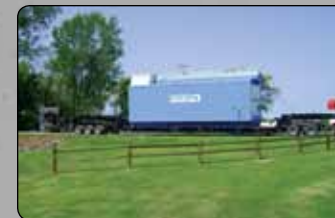
205,000 PPH with no burner shown on our 13 axle Cozad heavy-haul trailer.
