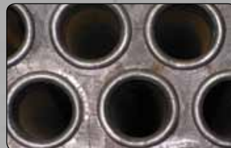
Tubes are rolled and beaded with a 3/4" to 7/8" ligament for maximum strength.
