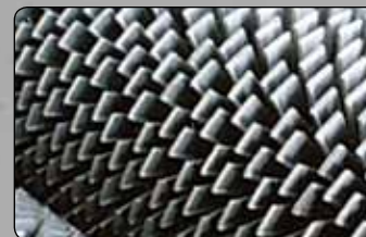
Serrated fins on a staggered tube layout are best suited for clean fuels.
