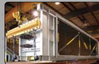
HRSG modules are designed for ease of lifting and movement.
