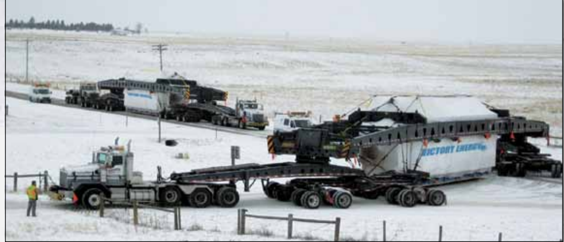
A pair of 220,000 PPH watertube boilers being delivered to Canada on special "perimeter-frame" trailers.
