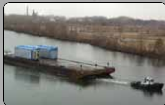
A pair of D-style boilers being shipped by barge.
