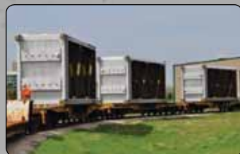
Three of six HRSG modules designed to ship by railway transport.
