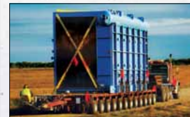
Waste heat HRSG being transported to a municipal solid waste job site.
