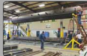
Beginning stages of the assembly process for a D-style watertube boiler.
